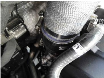
With the pipe now fitted to the engine, you will need to attach the two inlet ducts to the front end of the car. The forward facing ram-air duct will be attached to the front radiator support / slam panel using the original T25 Torx screws that secured the original intake ducting that were removed previously. The side duct is secured using the two T30 Torx screws that secure the upper edge of the radiator support just behind the headlight.
