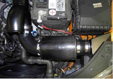
You will now attach the second carbon cannister using the remaining two 76-70 straight couplers. Due to the fixed nature of the pipe and the forward ram-air inlet duct, it will take some effort and manuevering to insert the cannister and attach both couplers to the piping. Once both couplers are attached to the piping, however, secure the hose clamps.
