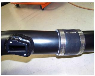
Now attach the piping assembly to the motor using a #70 hose clamp to attach the reducing coupler to the turbo inlet on the rear of the engine. If your vehicle is equipped with the noise pipe / engine amplification pipe, you may wish to remove this to give yourself more access to the hose clamps to attach the piping to the turbo inlet. Secure both hose clamps tightly.
