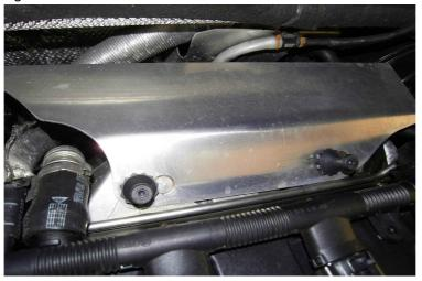
Using a T20 Torx bit, remove the MAF sensor from the OEM engine cover and fit this into the aluminium boss on the Forge piping using the two supplied 3mm Allen screws.
