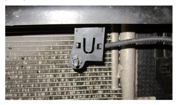
13. Now place your twintercooler between the upper and lower crash bar. You will need a paint marker pen or tippex to mark four points where you will drill 2mm-3mm holes .
