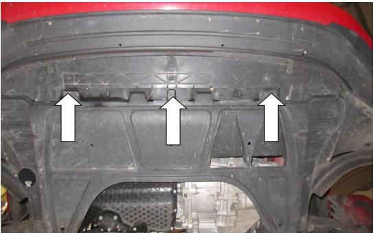
4. Pull down the arch liner, using your T25 Torx drive undo the fastener that attaches the bumper to the front wing .Then undo the two plastic nuts either side with your 10mm socket .As shown in the next picture.
