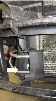
12. Disconect this temperature sensor on the lower side of the crash bar and bend the braket backwards. You will put this sensor on the mounting plate of your new Twintercooler once installed.
