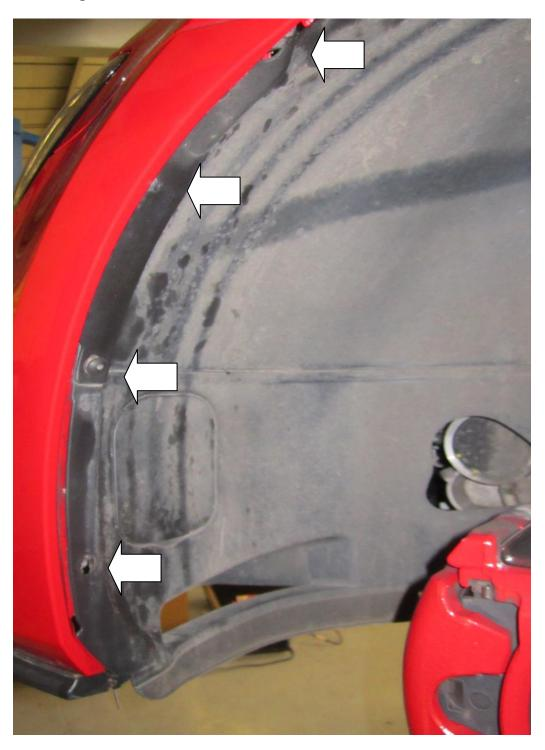
3. Again using your T25 Torx drive remove the fasteners from the undertray. This undertray can now be removed .
