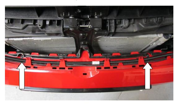
7. Now moving back to the sides of the car where the wing meets the bumper, pull towards yourself sharply to release the clips on the sides.
