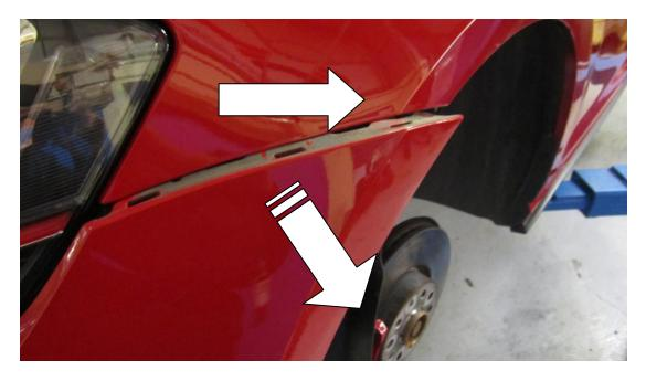
8. As you remove the bumper disconnect the loom to the fog lights and DRLs. Find a suitable container to catch the contents of your screen wash as this fitting also needs to be disconnected.
