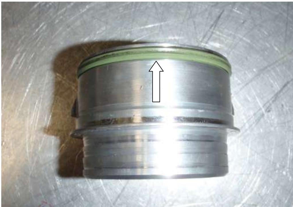
Drop the intercooler down and fit the male coupler into the intercooler, replace the clip and move up and down to ensure it locks in position. With the hose now in line move the intercooler up pushing the coupler into the hose, replace screws and tighten the intercooler. Position the JCS clip and tighten, replace the under tray and tighten all the screws. Installation is now complete!
