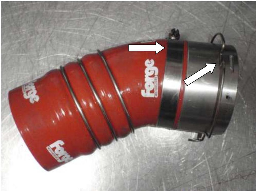
3. Carefully fit the coupler and hose in position taking care not to knock the clip out of position. Slide the clip up into the grooves of the coupler, move the hose/coupler up and down to lock into the grooves of the male coupler on the car. Push the intercooler up into its bolted position and rotate the hose around until it lines up with the inlet of the intercooler.
