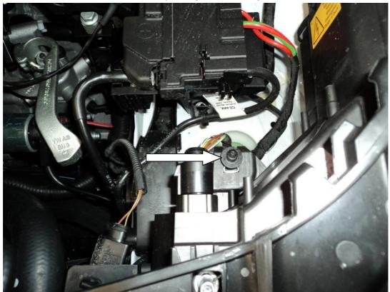
7. Using the bracket, solenoid, and the two 3mm Allen key bolts provided, place the solenoid onto the bracket and screw down, making sure the orientation is correct as seen in the picture below. Once this is done, connect the other end of the wiring loom onto the solenoid. Next, bolt down the bracket using the T30 Torx bolt removed from the headlight bracket previously.
