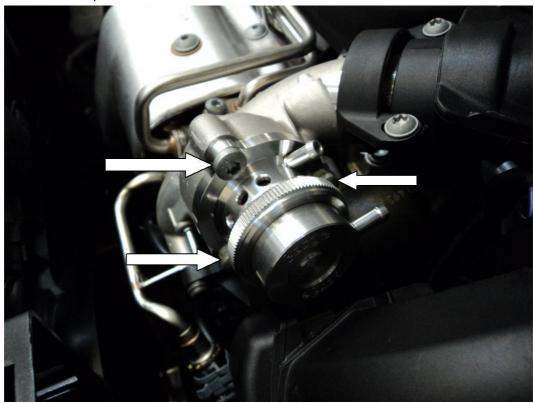
5. Using the plug you removed from the OEM valve, place this into the brown end of the wiring loom provided, making sure it clicks together.
