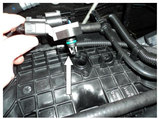
3. Push the new Forge aluminium vacuum take off block onto the bottom of the sensor, (this can be a tight fit), making sure the vacuum take off pipe is facing to the left (drivers side). Refit this back into the inlet manifold using the Phillip's headed self-tapping screws provided.
