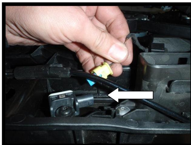
16. Unclip the large plug under the filter next to the outlet of the intercooler and unclip the remaining plug from the bracket.
