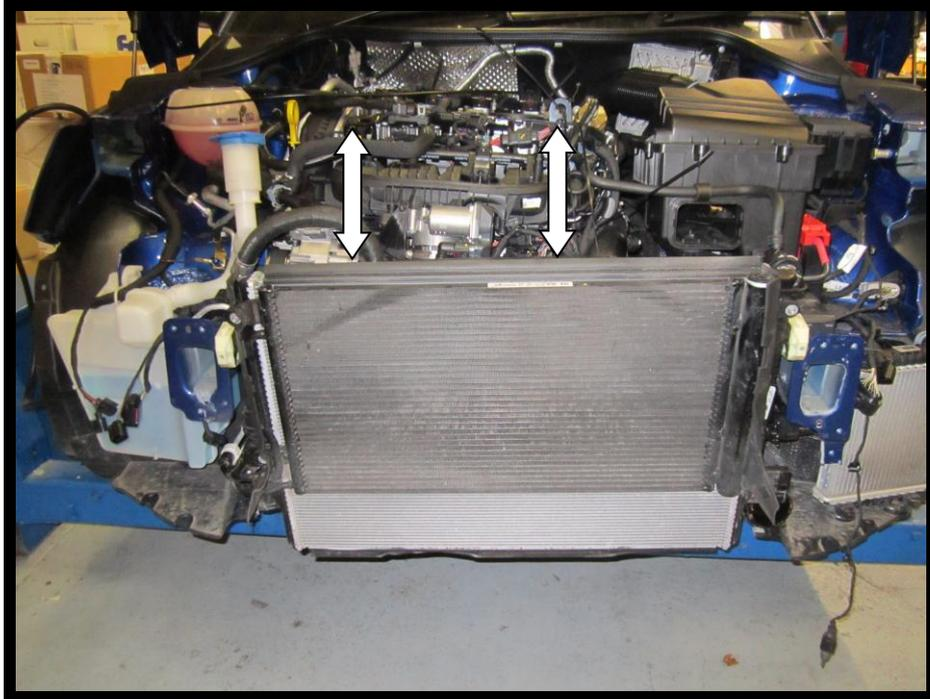
22. Once the radiator pack has been removed the remaining radiator and air condenser can be supported with a jack.
