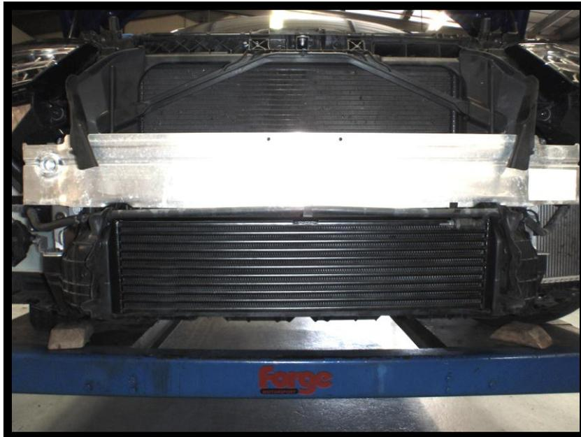
25. Making sure the intercooler is level with the radiator and crash bar, use a 6mm drill bit to drill a hole all the way through the bracket on the end tank and the rad pack. Using the nut bolt and washers supplied in the kit, secure the intercooler in position.
