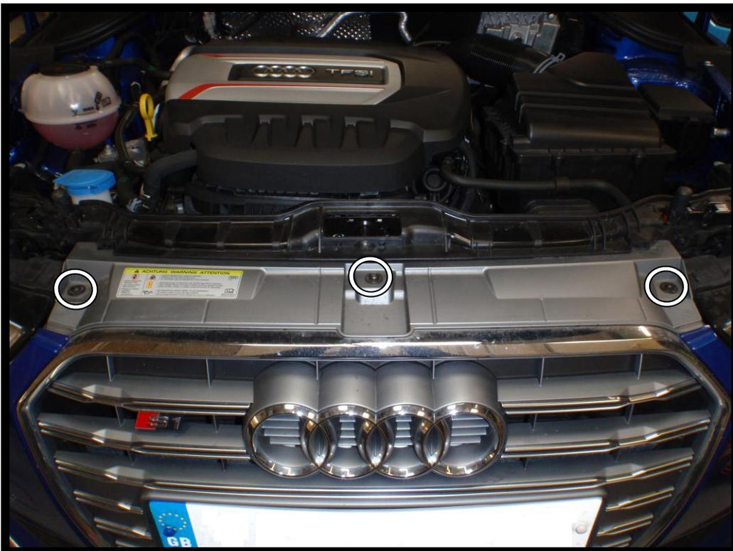
5. Remove the secondary radiator ducting by pushing it to the right until the clip is free.
