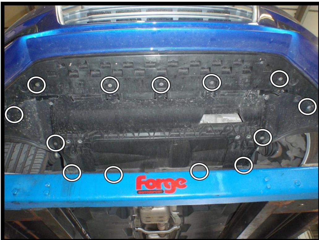
3. Under the arch liner in the corner of the bumper is a small plastic clip. Remove with a flat bladed screw driver, then carefully pull the bumper out of the clips of the wing.
