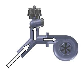
Symmetrical mounting of the turbo and wastegate is excellent for boost control, but not always possible upon installation due to space constraints
