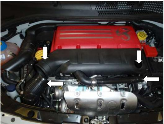
2. Remove the dipstick and using a T20 screwdriver, remove the MAP sensor from the inlet manifold. You may find it easier to remove the screw holding the fuel pipe in place to give you a bit more access.
