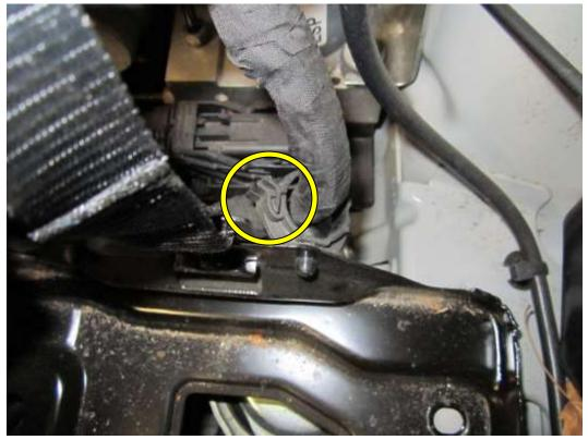
11. Now the battery tray has been completely removed locate the sensor that mounts on the boost pipe beneath, Using a T25 torx drve remove the sensor.
