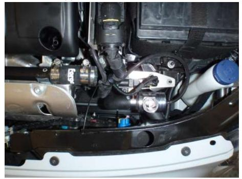
20. Finally, plug the supplied wiring plug into the solenoid, and into the factory plug you removed from the stock valve in step 5. Installation is complete (note wiring may vary from illustration below)
