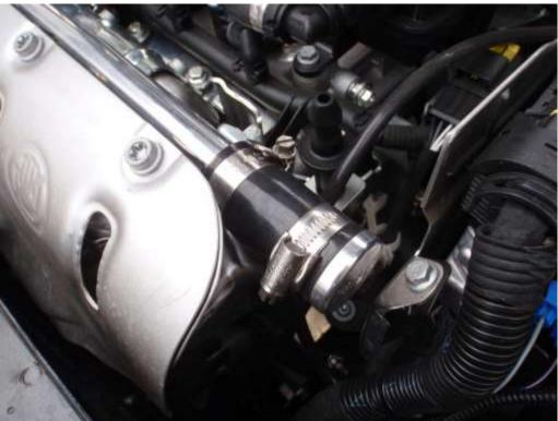
19. Offer the valve up to the bracket already fitted, and pull the lower rubber hose through the jubilee clip welded to the bracket, and push it over the base pipe of the valve. Tighten the clip to secure the valve and pipe to the bracket.
