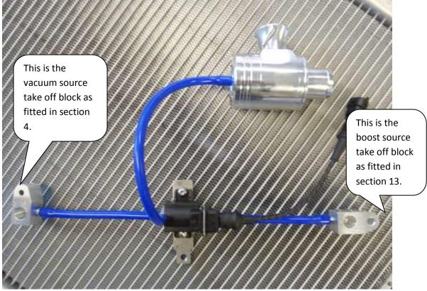
17. You now need to decide if you want a noisy or quiet valve. The side pipe of the valve can be changed for noisy (trumpet) or quiet (tube). Simply unscrew and screw on which ever you want.
