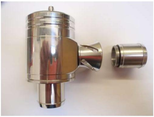
18. If you want a NOISY valve connect the trumpet to the valve, and the supplied short length of silicon hose, Forge banking plug and jubilee clips to the small pipe on the front of the engine cover to blank it off(shown with the Forge induction kit). For a QUIET valve, just reuse the stock rubber hose between the engine cover and the dump valve, with the tube on the side of the valve.
