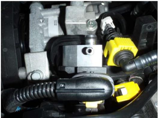
4. Connect the supplied length of silicon vacuum hose to the takeoff just fitted, and route it around the engine bay, using the clips already on the bulkhead to hold it in place, and route it between the ECU and the engine block to the front of the car by the stock valve. Use the supplied cable ties to secure it in the engine bay.
