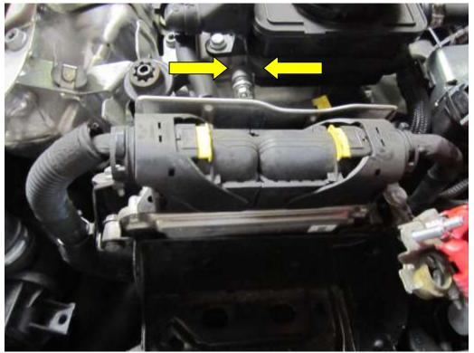
10. There are several plastic clips on the battery tray these need to be un clipped to remove the tray completely ,Do this by pulling back on the tab as pictured .
