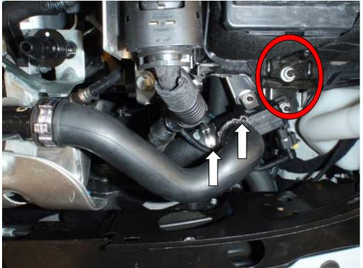
6. You must now remove your battery and battery tray to gain access to your boost source. Using a 13mm Ratchet and extension remove the 13mm nut circled in red.
