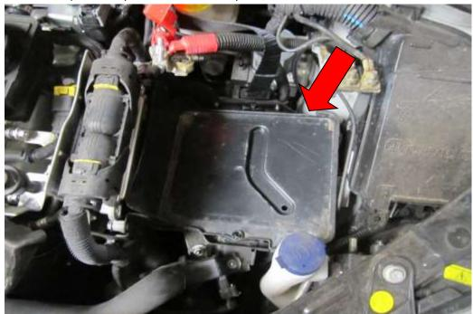
7. Pull out the plastic tray beneath the battery .
