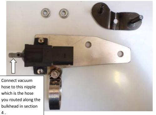
16. Then connect the other vacuum pipe to the solenoid that comes from your boost source, This is the piece of vacuum pipe you fitted to the take off block beneath your battery tray the image below shows you the correct way to install all your vacuum pipes .
