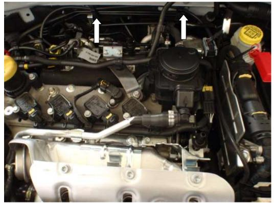
5. Remove the two clips arrowed below that connect the stock valve to the engine. Remove the electrical connector by pulling out the yellow 'safety' catch and then squeezing the connector to pull it off. Remove the two 10mm nuts holding the valve to the bracket on the chassis – MAKE SURE you have a hand under the valve to catch the bracket as it falls off !
