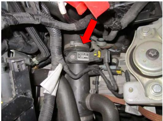
12. Place the boost take off block under the sensor and refit using the longer screw provided .
