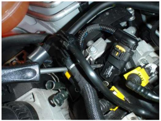
3. Place the Forge vacuum take off under the MAP sensor and push it securely in place, ensuring the o-ring is fitted to the take off. Screw the takeoff and MAP sensor as one unit back to the inlet manifold with the provided brass screw.
