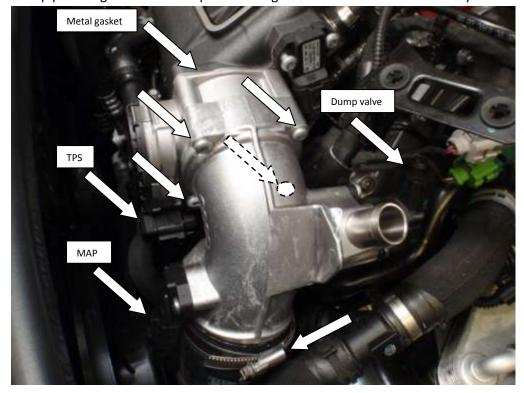
3. Attach the throttle body with the new o ring supplied in the kit. Also attach the MAP sensor with the existing bolts.
