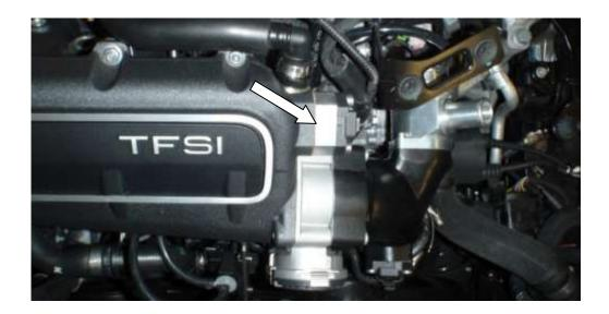
8. Forge highley recommend venting to atmosphere as this valve has a bigger bore for releasing the boost pressure. However you can install this valve recirculating if you wish. Follow step one in reverse order and your installation is now complete.
