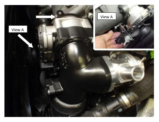
5. This photo shows the how to connect the vacuum pipe assembly.
