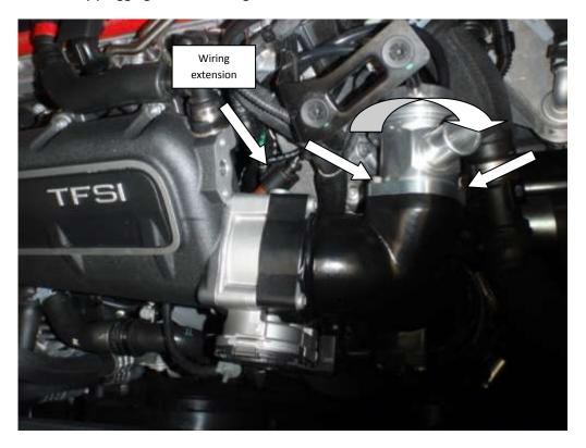
7. Bolt on the vacuum take off block using the bolts and gasket supplied, The port needs to be facing down, connect the solonoid to the dump valve as shown in step 5 with the vacuum hose passing under the inlet mainifold.
