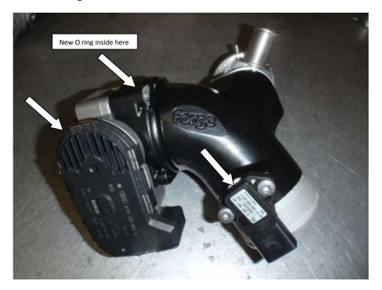
4. Refit the high flow inlet pipe with dump valve in reverse order of step 2. Take care when refitting the metal gasket and bolt on the solenoid as shown in view A.
