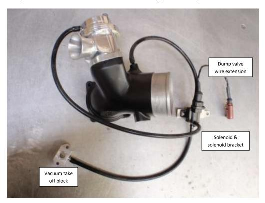
6. If there are any clearance issues when the high flow inlet and dump valve is fitted. Remove the dump valve with a 5mm allen key, on the base of the flange you will see two small bolts undo with a 3mm allen key. Rotate to the appropriate position and reattach dump valve. Push the dump valve plug under the oil filler cover bracket and wires .Connect to the solonoid by plugging into the wiring extension.
